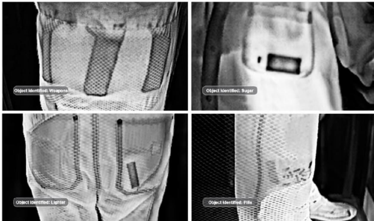
The Mini Portal's infrared camera detects heat radiating from even a tiny object, producing a shape on the image. It is irrelevant how long an object has been concealed under clothing as a new temperature imprint is created every time it is scanned. Infrared rays don't penetrate beyond the clothing so passenger privacy is protected.
